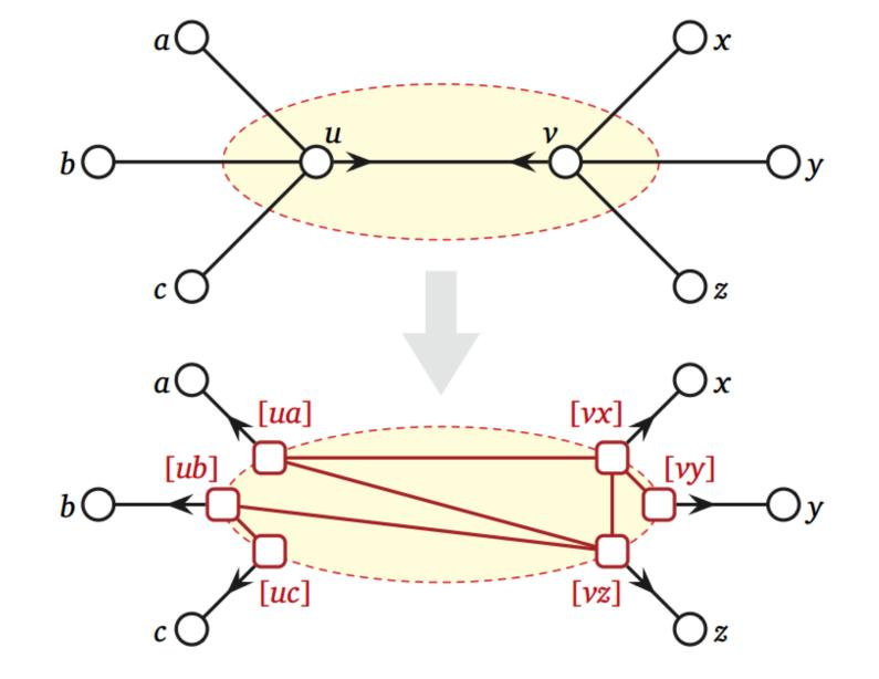
**Figure 2.** An example of edge expansion. An arrow leaving a node indicates the base of that node.
