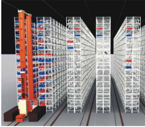
(a) An AS/RS with storage racks and aisle-based S/R machines
