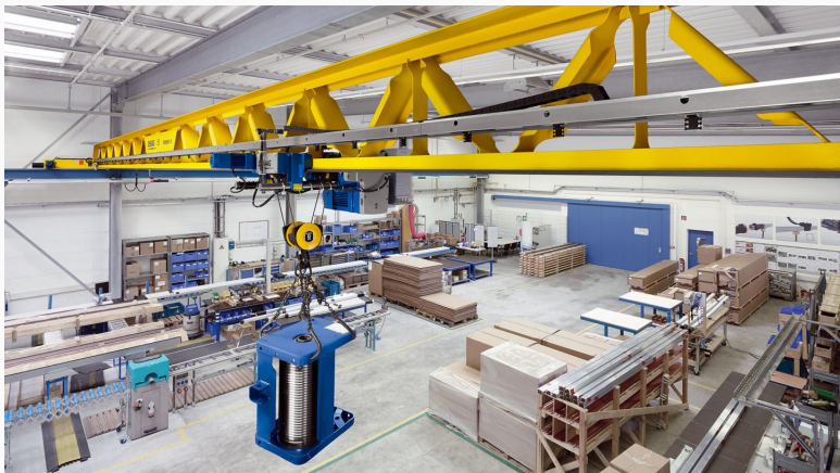
Figure 1: Demag V-type crane machine. Source: demagcranes.com
